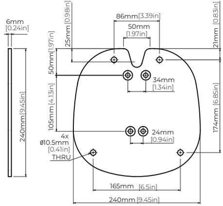
**Important!** No more than 100kg (220lbs) should be mounted above 1.2m (47.25") on a single column.
