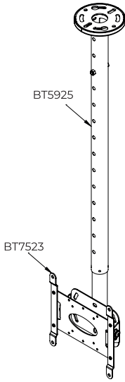
Single Screen Installation
