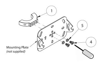
\*Important: Ensure to fix the mounting plate to the front half of the collar (item 1).
