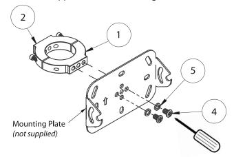
\*Important: Ensure to fix the mounting plate to the front half of the collar (item 1) so you have access to item 3 on the back.
