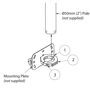
iii. Position collar on pole and fasten *item 3* tightly ensuring the gap between the collar halves on both sides are equal.
